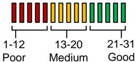
Note: Reception levels below 14 can give problems with the relay operation, and poor quality audio, or no audio coming from the microphone on the intercom (the person on the phone cannot hear anything), or buzz on the loud speaker.
