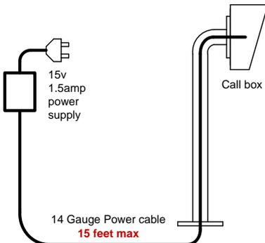
**Tip:** 18 gauge cable will not run the unit. You may experience various issues with performance if the power cable is more than 15 feet and using thin cable such as 18 gauge.
