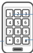
Press # key to **LATCH** output relay. Caution: Use only for holding open gates or door!.
