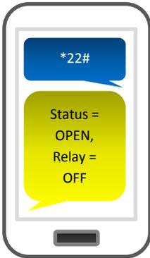
Send the SMS as shown, and the unit will reply showing the status of the input limit switch (if used), and the relay..
